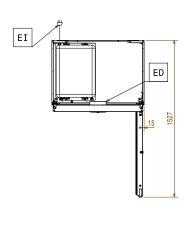
**Electric** Supply voltage: 220-240 V/1 ph/50 Hz Electrical power, max: 0.45 kW Capacity: Number and type of grids (included): 5 - 530x700 **Key Information:** Net Volume: 510 It Door hinges: External dimensions, Width: 900 mm
